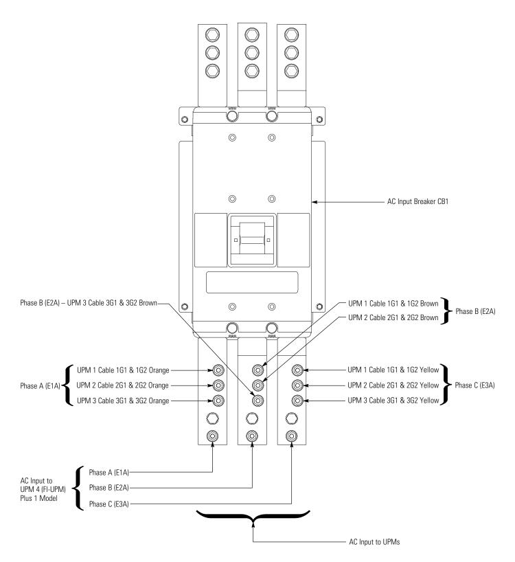
**NOTE** Two cable lugs will be connected to each terminal stud. When connecting the cable lugs, install the first lug on the stud with the raised barrel portion facing the back of the cabinet. Install the second lug with the raised barrel portion facing the front of the cabinet.
